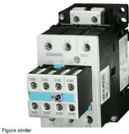
CONTACTOR, AC-3 22 KW/400 V, AC 220V 50HZ/240V 60HZ 2 NO + 2 NC 3-POLE, SIZE S2, SCREW CONNECTION
